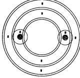
Fig. 4 Use of the 5.6 mm (.22 in) gauge on OUTWARD gauging targets (Rule 5.1.7)
